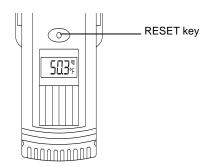
**NOTE**: Do not use sharp objects to press the RESET key. Use a small dull pointed object or a straightened paper clip and **gently** press the RESET key to commence NORMAL MODE.
